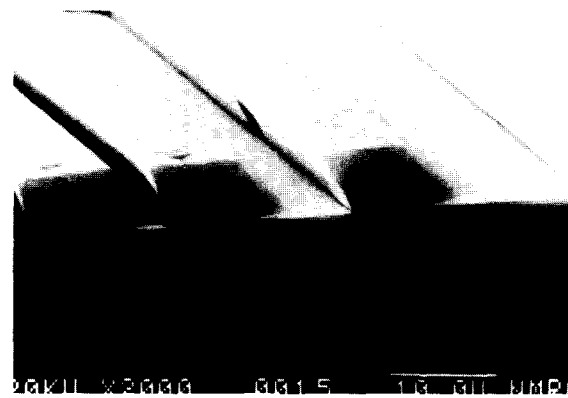
Figure 14 The 10, 5 and 2\ \mu\text{m} lines in 6\ \mu\text{m} thick resist layer showing good undercut. The undercutting is necessary for processes involving 'metal lift-off' and is achieved by over-exposure
